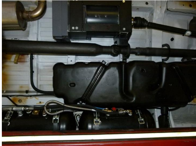
Generator and air tanks under the car
